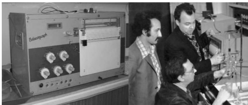
Fig. 5 Recording polarograph, Model OH-102, Radelkis, Hungary. This polarograph allowed normal and derivative modes of polarography. PhD student Evgeny Katz (standing, left ), Dr. Yuriy Kozlov (standing, right ) and Prof. Boris Kiselev ( sitting ) performing measurements with Polarograph OH-102 (Institute of Photosynthesis, Russian Academy of Sciences, Pushchino, 1977)
