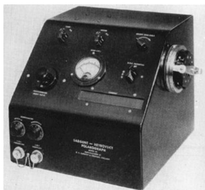
Fig. 3 Sargent–Heyrovský photographically recorded polarograph Model XII manufactured by EH Sargent and Co., Chicago (Courtesy of ACS)
